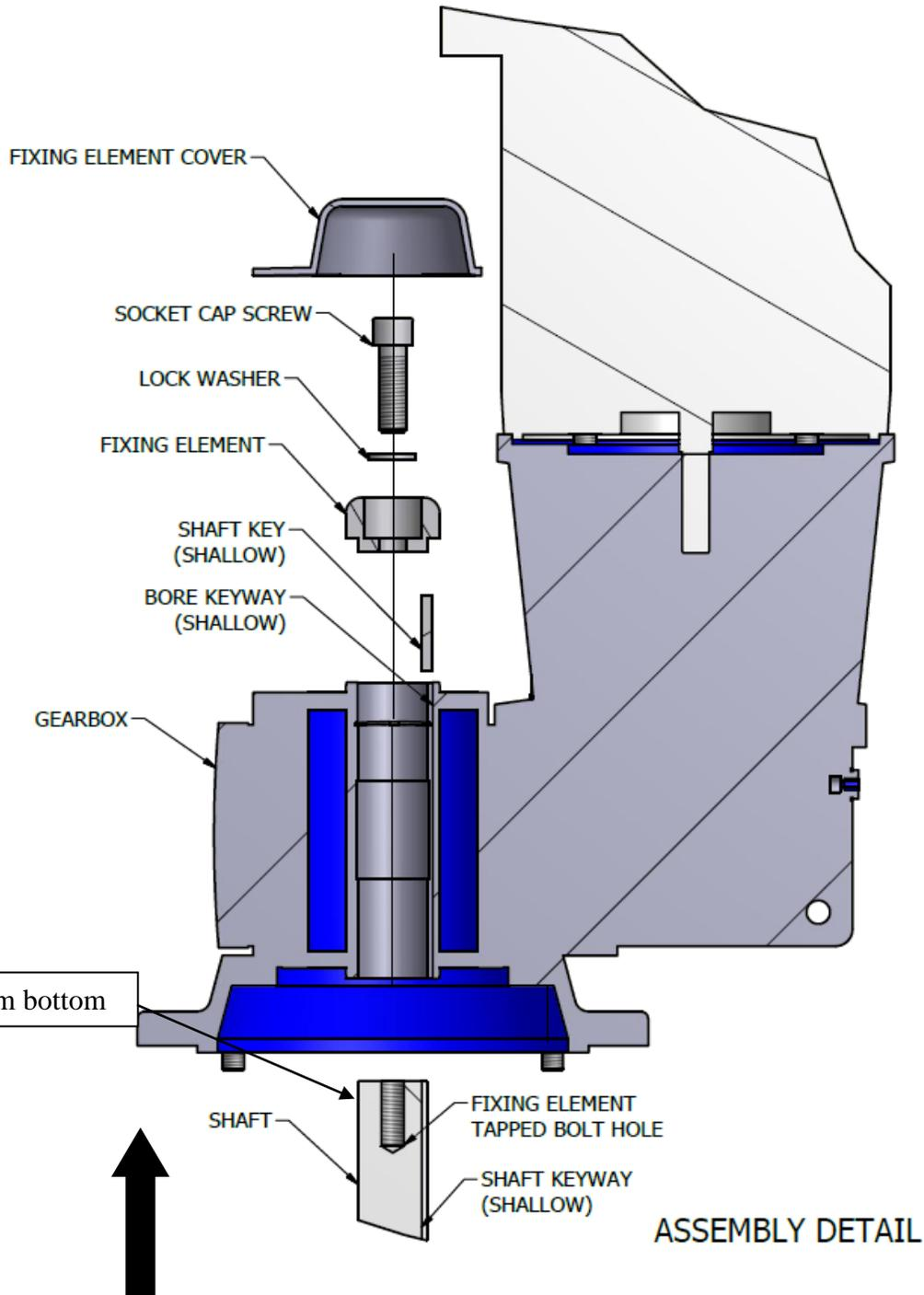
Step 6: (See Bulletin 02-200 for illustration) Remove turbine/turbine hub from packing and slide hub over shaft end until above keyway. Insert key and lower hub into position. Tighten hub set screws into key and shaft.
