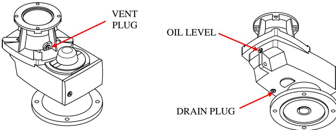
**NOTE:** For NEMA 250TC and larger standard Perma CLASSIC lubrication system will exist. Please change system according to plug in end of lubricator.
